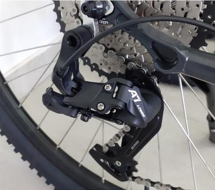
The gears on the bike should be used with care, as the power of the motor can damage the gearset. When using the gear shifter, it is important to reduce pressure on the pedals. **DO NOT** shift the gears under full pedal load. **DO NOT** shift gears without pressing the pedals.
