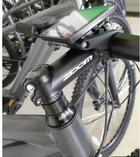
The Zoom stem with a length of 100 mm and a 5° rise provides better control of the bike at higher speeds and on rough terrain.
