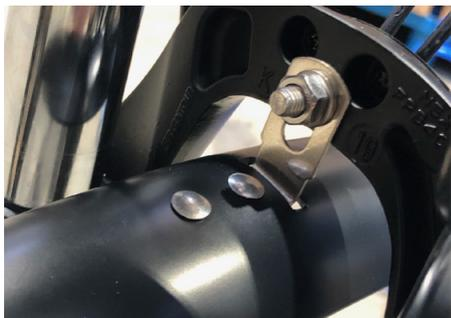
First, remove the fork protection. Insert the fender brackets (two aluminum rods) into the plastic holders attached to the bike's fork and tighten the screws on the sides using a 3mm Allen wrench. The fender has a hook through which you insert the screw and tighten it together with the light into the opening on the fork. When tightening the screw, make sure the light is facing upwards.
