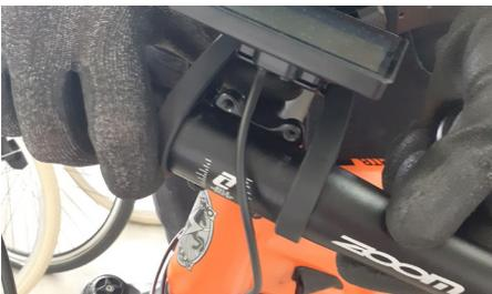
Cut the ties securing the handlebar to the bike, remove the handlebar protector and the protector from the handlebar stem
